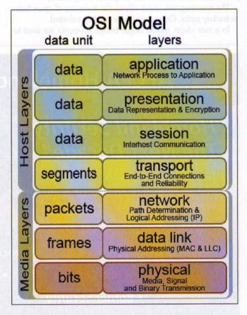
The open systems interconnection model layered approach, shown in this table, allows each subordinate, interdependent layer to provide services to the next higher layer as transactions are converted from lower to higher abstraction levels. Each layer, sending messages as binary bits, is interdependent; if a layer is compromised, the other layers will not know, causing Global Information Grid communications to cease.
