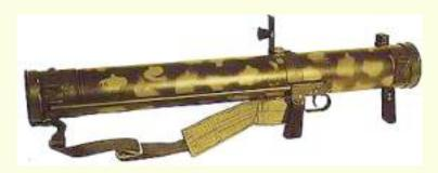
The RPO-A (Recoilless Infantry Flame Thrower) *Shmel* ("bumblebee"), is a single shot, disposable, lightweight, shoulder-fired, recoilless "rocket" launcher. Designed to kill personnel in dug-in and covered fighting positions, buildings and shelters.
